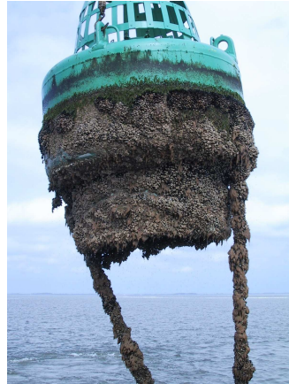
Reference buoy without anti-fouling protection
